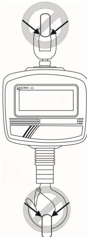
**Do not use too large load attachment devices which cannot guarantee a one-point suspension.**
