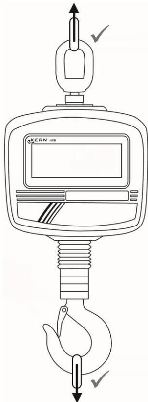
**Only use load attachment devices which guarantee a one-point suspension and where the scales can be suspended freely.**
