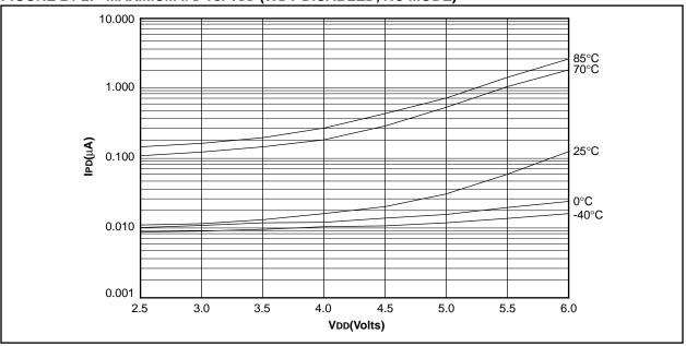
FIGURE 24-3: TYPICAL IPD vs. VDD @ 25°C (WDT ENABLED, RC MODE)
