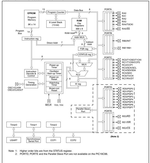
FIGURE 3-4: PIC16C66/67 BLOCK DIAGRAM
