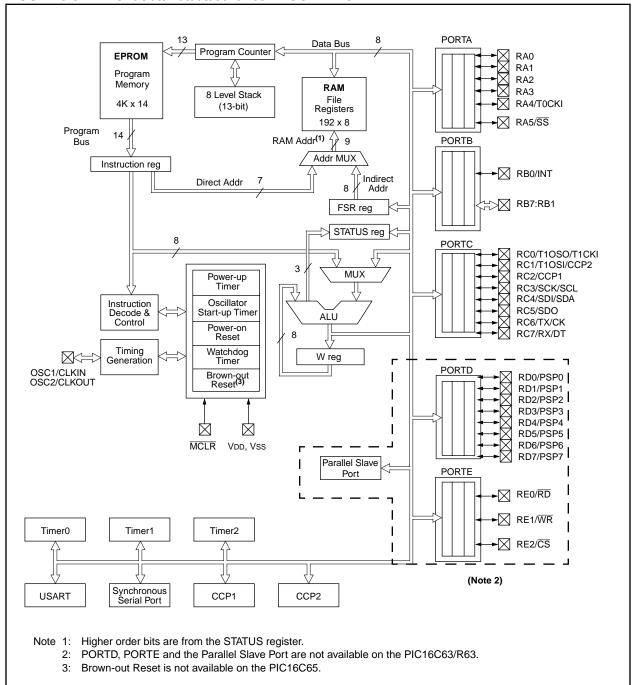
FIGURE 3-3: PIC16C63/R63/65/65A/R65 BLOCK DIAGRAM
