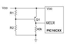
Note 1: This brown-out circuit is less expensive, albeit less accurate. Transistor Q1 turns off when VDD is below a certain level such that:
