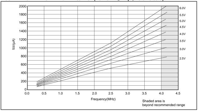
FIGURE 24-14: TYPICAL IDD vs. FREQUENCY (RC MODE @ 100 pF, 25°C)
