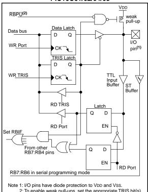
2: To enable weak pull-ups, set the appropriate TRIS bit(s) and clear the RPBU bit (OPTION<7>).
