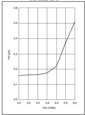
FIGURE 17-6: TYPICAL IPD VS. VDD WATCHDOG TIMER ENABLED 25°C
