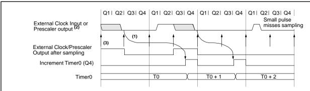
Note 1: Delay from clock input change to Timer0 increment is 3Tosc to 7Tosc. (Duration of Q = Tosc). Therefore, the error in measuring the interval between two edges on Timer0 input =  $\pm 4$ Tosc max.
