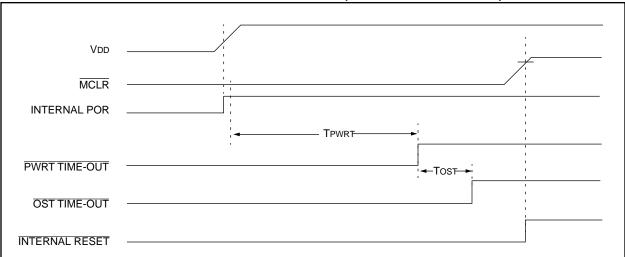
FIGURE 13-13: TIME-OUT SEQUENCE ON POWER-UP (MCLR TIED TO VDD)
