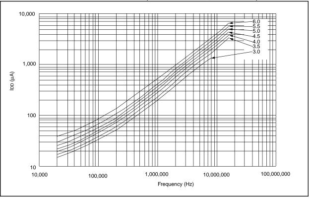
FIGURE 17-14: MAXIMUM IDD Vs. FREQUENCY (EXTERNAL CLOCK, -55° TO +125°C)
