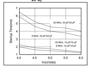
FIGURE 24-24: TYPICAL XTAL STARTUP TIME vs. VDD (XT MODE, 25°C)
