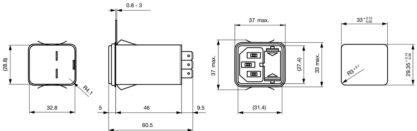
Screw-on mounting from front side with ground line choke
