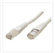
Patch cable for networking connections between devices. Prepared double shielded Twisted Pair cable with screened RJ-45 connectors on both ends. Durable due to moulded kink protection. Flexible cable, suitable for narrow bending. High quality plugs with gold plated contacts. Contact settings 1:1, in accordance with the EIA/TIA 568 standard. Construction: 4-pair stranded copper wire. Complete braid shielding. Pairs shielded with aluminium clad polyester foil.
