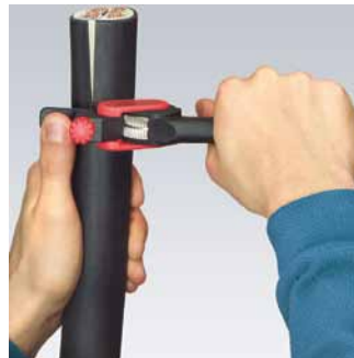
Turning the tool for circumferential cut
