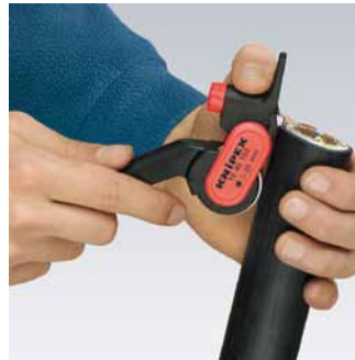
Setting the tool for longitudinal cut
