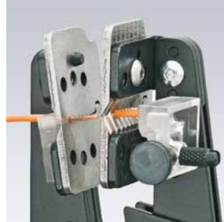
The precise shape of the blades leads to perfect stripping
