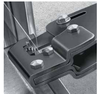
The punching tool is squeezed through the metal section sheets
