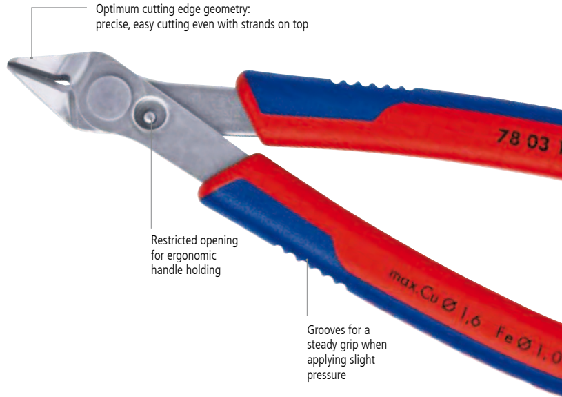
78 03 125 / 78 23 125 INOX-stainless steel; cutting edge hardness approx. 54 HRC
