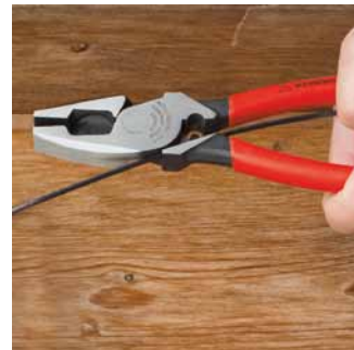
09 11/12 240: Fish tape puller in the joint gap
