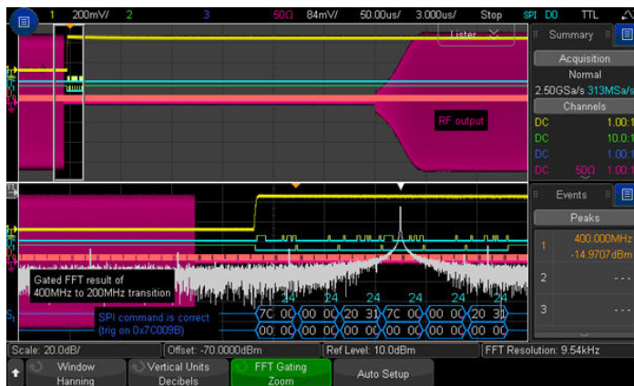
Figure 21a. Triggered on a SPI command, the RF signal is still at 400 MHz as indicated in the frequency peak search result list.
