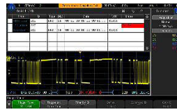
Figure 17. CAN-FD decode and trigger.
