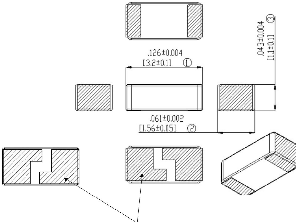
1. Antenna is symmetrical, both of antenna pattern have same RF performance.
