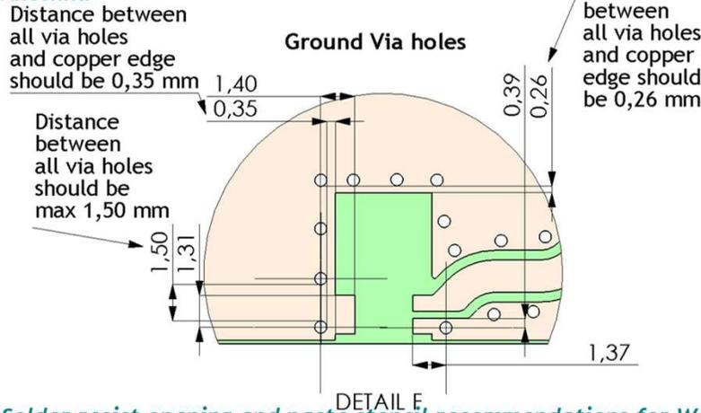
*Solder resist opening and paste stencil recommendations for W3020 US-WiMax Antenna*
