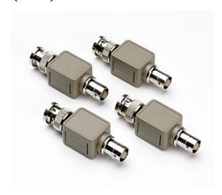
The TA050 attenuator set consists of four coaxial attenuators designed for use with signals up to 1 GHz. Each attenuator has a male and a female BNC connector.
