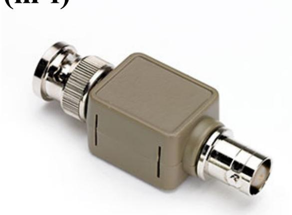
The TA051 feed-through attenuator is a coaxial terminator with BNC connectors. It is useful for connecting signals from 50 Ω sources into instruments with 1 MΩ impedance inputs, such as oscilloscopes.
