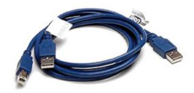
The TA146 is a high-quality 1.8 metre USB 2.0 Y-cable designed and built specifically for use with PicoScope oscilloscopes, and featuring 20 AWG conductors for minimal resistance. This also reduces the chance of voltage drop caused by inferior USB ports on some PCs and laptops. As well as reducing voltage drop, it prevents noise that could be caused by an unreliable ground connection and poor screening in inferior cables.
