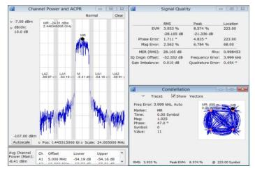
SignalVu-PC application SV26 enables quick, standards-based transmitter health checks on APCO P25 signals. The following image shows a Phase II signal being monitored for anomalies with the spectrum analyzer while performing transmitter power, modulation and frequency measurements.
