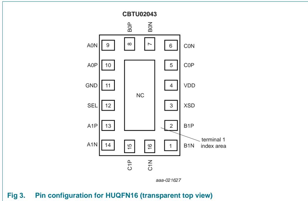
**Fig 3. Pin configuration for HUQFN16 (transparent top view)**
