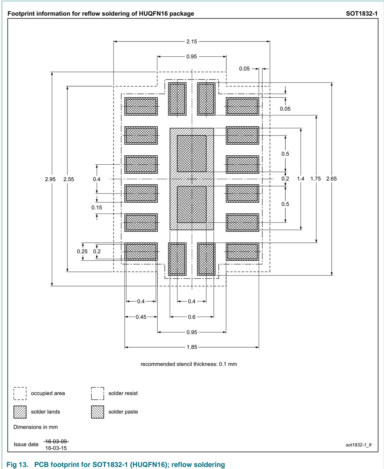
Fig 13. PCB footprint for SOT1832-1 (HUQFN16); reflow soldering
