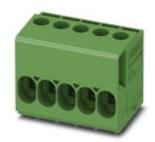
PCB terminal block, nominal current: 24 A, nom. voltage: 400 V, pitch: 5.08 mm, number of positions: 5, connection method: Screw connection with tension sleeve, mounting: Wave soldering, conductor/PCB connection direction: 0 °, color: green
