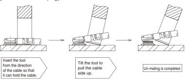
Never un-mate the plug by pulling the cable. It may cause a failure of the connector.
