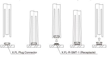
(2) Allowable load to a cable that is mated
