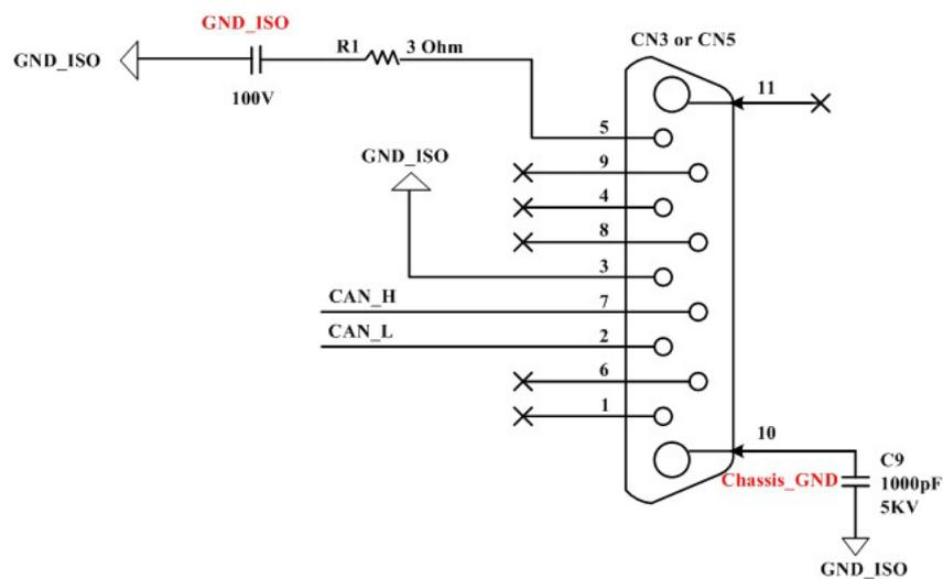
Figure 4.2 PCIe-1680 DB-9 connector schematics
