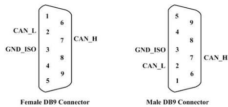
Figure 4.1 PCIe-1680 DB-9 connector pin assignments
