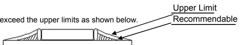
Accordingly increasing the solder volume, the mechanical stress to product is also increased. Exceeding solder volume may cause the failure of mechanical or electrical performance.
