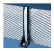
The right angle base in black accepts a flat cable width of 2.0" (50.8 mm) and is made of nylon 6.6, which increases mechanical strength, heat and wear resistance, and stiffness. It is designed for indoor environments.
