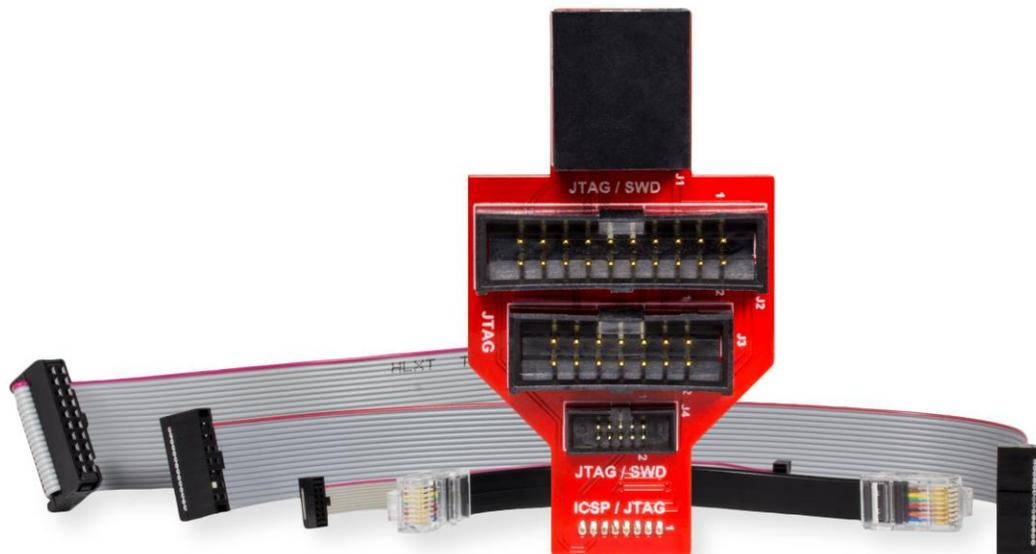
**ICD4 RJ45 Universal Adapter Board**
