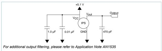
Figure 5. Recommended power supply decoupling and output filtering
