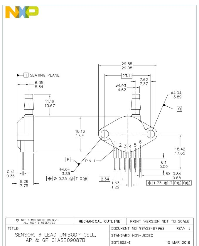
0 to 250 kPa, Differential, gauge pressure sensor, on-chip signal conditioned, temperature compensated and calibrated
