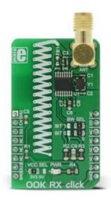
**OOK RX click** is a wireless receiver that operates at the frequency of 433MHz (sub-GHz). This device allows realization of a simple, low-speed wireless ad hoc communication network between a receiver and compatible transmitter. This device features an ASK/OOK demodulator, analog RSSI output, and integrated squelch capabilities.
