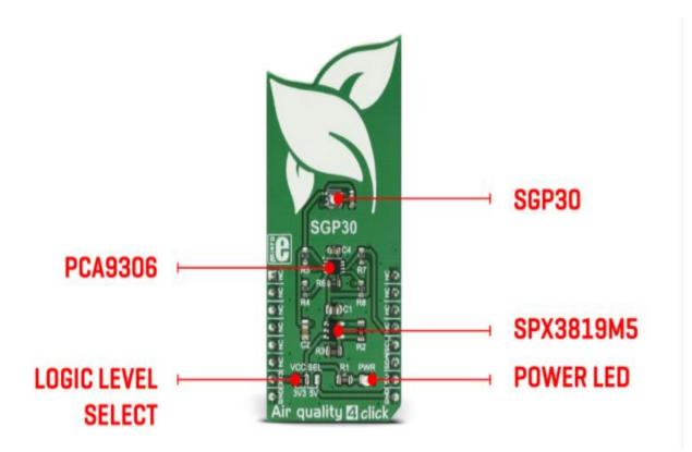
The device also allows air humidity corrections over the results for both the compensated and raw values. However, an absolute humidity sensor should be used for obtaining the humidity reading. Readings from SHT click or any other similar humidity measuring device can be used for this purpose. The appropriate I2C command will store the value into the on-chip memory and perform the corrections, accordingly.
