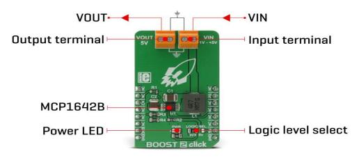
The MCP1642B-ADJ step-up regulator actively damps the oscillations typically found at the switch node of a boost converter. This removes the high-frequency radiated noise, ensuring low noise operation.
