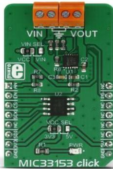
The click operates with the input voltage range from 2.7V up to 5.5V and it is capable to deliver a regulated output ranging from 0.8V to 3.5V, with up to 1.2A. The output voltage is selectable and it is managed by the voltage on the FB pin. This pin is routed to the output of the [MCP4921](#), a 12bit DAC converter from Microchip, with the SPI interface. The voltage on the DAC output affects the FB pin voltage, which in return affects the main output voltage.
