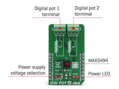
All the communication with the control logic of the MAX5494 is done through the SPI, so all the SPI signals are routed to the appropriate mikroBUS<sup>™</sup> pins. The CS pin is held high, preventing the SPI communication, so as always - to initialize the SPI communication, the CS pin needs to be pulled LOW by the MCU.
