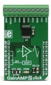
The rail-to-rail inputs and outputs accept voltage levels up to VCC with no distortions or phase shifting. The output voltage is offset by the resistor ladder network on the output stage and the voltage on the voltage reference pin.
