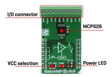
Besides the VOUT pin on the 10 pole I/O connector, the MCP6S21 output pin is also routed to the AN pin of the mikroBUS™ so it can be used as the input signal for the ADC. This allows the amplified signal to be easily digitalized and processed by the MCU. Using the click board in this configuration effectively turns the GainAMP 2 click into an analog port expander with the selectable gain on its inputs.
