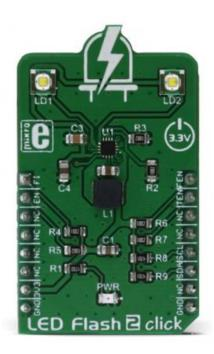
The click board comes equipped with the two XPCWHT-L1-R250, high brightness LED elements by Cree, Inc.
