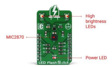
Flash inhibition pin, or the FI pin - routed to the mikroBUS<sup>™</sup> AN pin, with the corresponding bit in the Torch control register (02h), is used to limit the Flash mode current value to the Torch mode current value. This will effectively override the Flash mode.
