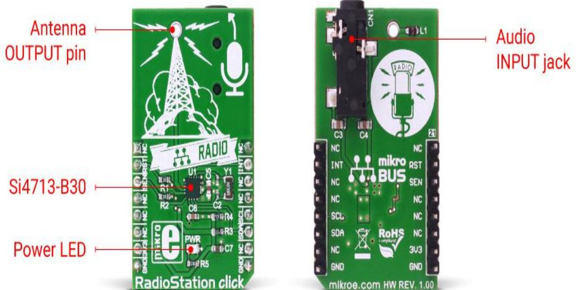
The click is designed for communication over the I2C/2-wire control interface. When selecting 2-wire mode, SCLK pin should stay at a HIGH logic level during the rising edge on the RST pin, and stay HIGH until after the first start condition. Also, a start condition must not occur within 300ns before the rising edge on the RST pin. The 2-wire bus mode uses only the SCL and SDA pins for communication.
