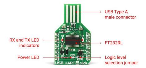
This device also features the configurable CBUS pins, which can be used for several different useful functions, as for example - configurable clock out for driving the microcontroller, data LED drive, USB Sleep, PWR status and so on. By default, CBUS3 and CBUS4 pins are configured as Power Enable and Sleep options and are routed to the PWM and RST pins of the mikroBUS<sup>™</sup>, respectively. More information about configuring the CBUS pins can be found in the FT232RL datasheet.
