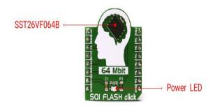
When configured to work in a regular SPI mode, the SQ2 and the SQ3 pins will become Write Protect function and Hold function pins:
