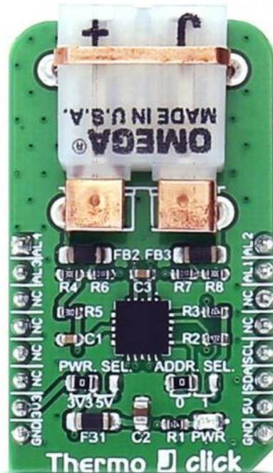
To obtain the desired measurement of the temperature, the cold end temperature needs to be known, too. Since the MCP9600 features an integrated measurement of the ambient temperature (cold junction compensation), error corrected value can be read directly from the registers, using the I2C bus protocol.
