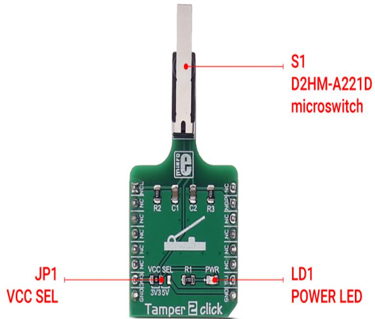
The switch itself is very durable and its rated up to 42VDC / 0.5A, also can endure a very high number of switching cycles – up to 1000000.
