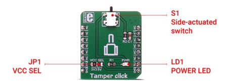
The used switch itself is intended to operate with digital signal levels, thus its electrical characteristics are tailored for this purpose: low contact resistance of  $100m\Omega$ , relatively low contact ratings of 100mA at 12V and 50 000 switching cycles before the failure. These attributes make it ideal for digital signal applications, specifically.
