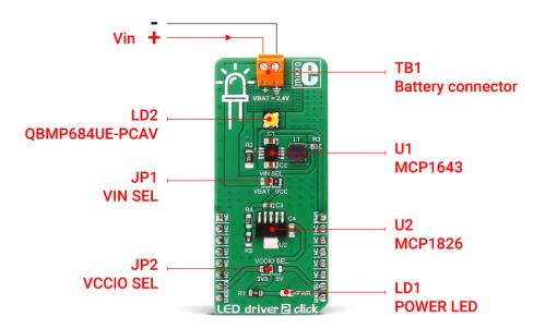
The LED brightness can be regulated by applying a variable duty cycle PWM signal to the EN pin of the MCP1643 regulator (routed to PWM pin on the mikroBUS<sup>TM</sup>). This results in changing the current running through the LED in a linear fashion, from 0 to the value set by the resistor, depending on the PWM cycle.
