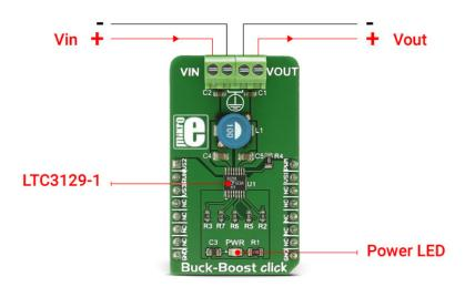
Buck-Boost click is able to work in two different modes of operation, depending on the nature of the application it is used in - PWM mode and Burst mode.
