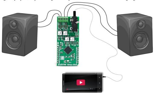
The output of the modulator is used to gate the output transistors on and off, alternately. The high efficiency of a Class D amplifier is due to the switching operation of the output stage transistors. Since the transistors are either fully ON or fully OFF, they spend a small amount of
