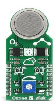
Note: The click carries TXB0106 Voltage Translator. For selecting the interface voltage level, use the onboard jumper, and choose between the 3.3V and 5V. For more information, see the Jumpers and Settings table below.
