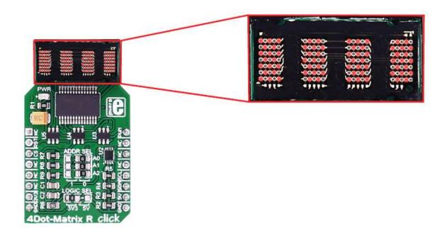
SLO2016 is a 4-Digit 5x7 Dot Matrix Alphanumeric **intelligent display**, with many built-in functions that will save your time. The integrated circuit contains memory, a 128 ASCII ROM decoder, multiplexing circuitry and drivers.
