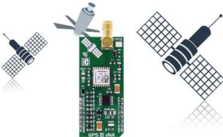
The user wanting to use GPS to determine its position must have an antenna that receives the signals coming from the satellites, and a receiver that translates these signals. The antenna position will be deduced from the measurements of the time delay between the emission time (satellite) and the reception time (receiver) for at least 4 signals coming from different satellites.
