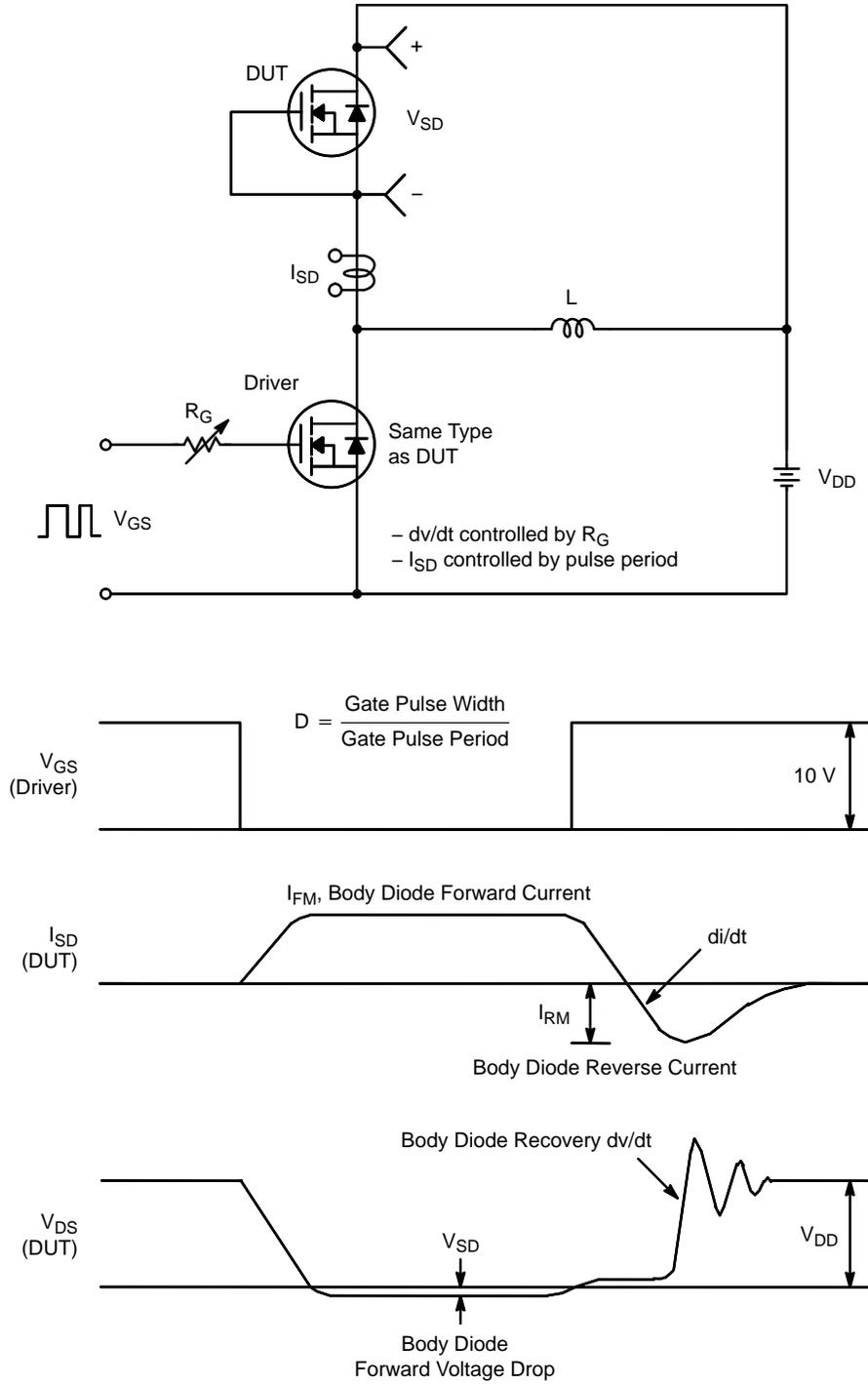
**Figure 16. Peak Diode Recovery  $dt/dt$  Test Circuit & Waveforms**
