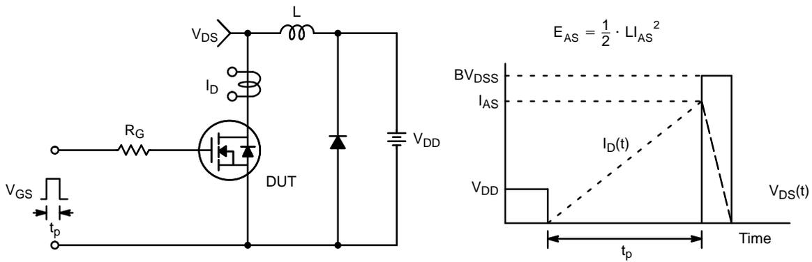
Figure 15. Unclamped Inductive Switching Test Circuit & Waveforms
