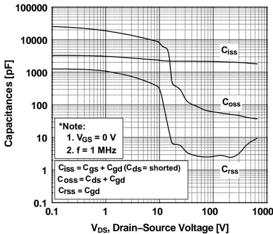
Figure 5. Capacitance Characteristics
