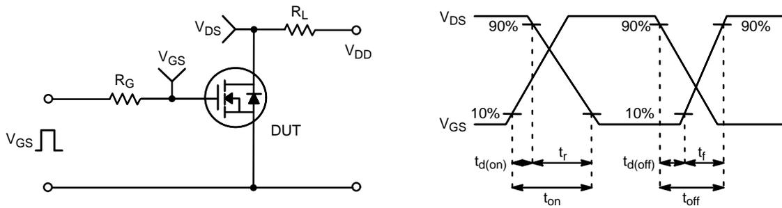
Figure 14. Resistive Switching Test Circuit & Waveforms
