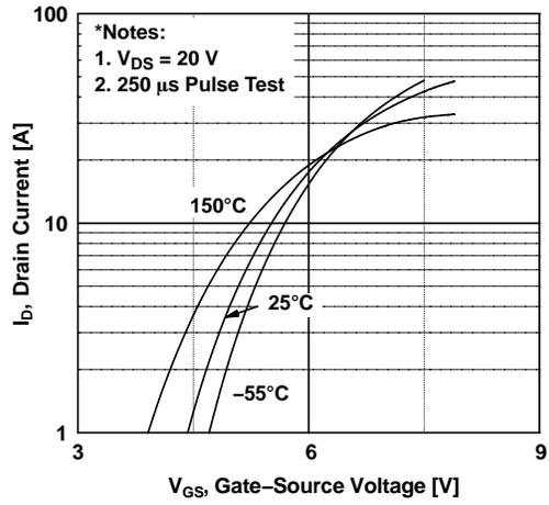
Figure 2. Transfer Characteristics
