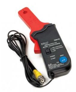
The TA018 current probe can measure currents from 10 mA up to 60 A with a switch-selectable high and low range. A simple pushbutton is included for zero adjustment when measuring DC current.
