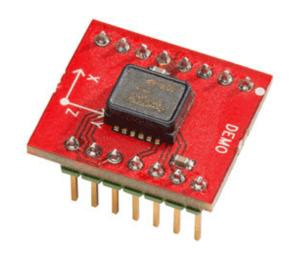
Sensor Boards for Degital Accelerometers
