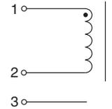
\*Pin 3 is for mechanical support only and has no internal electrical connection
