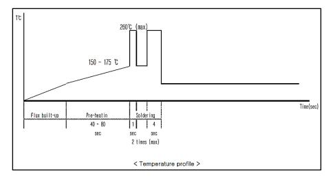
■ The temperatures defined above are the temperatures measured on the surface of the Printed Circuit Board. There are cases where the printed circuit board's temperature differs greatly from the temperature of the switch. Critical note: the switch's surface temperature must not exceed 260°C.
