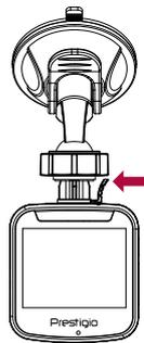
1. Attach the bracket to the device. Slide and push until the connection is firm.
