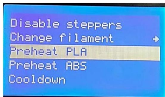
Preheat the nozzle before feeding and retreating, quickly pull out the filament after the filament is withdrawn, otherwise the filament will block the nozzle.
