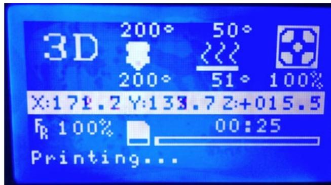
(On the top is the preset temperature, on the button is the actual temperature)
