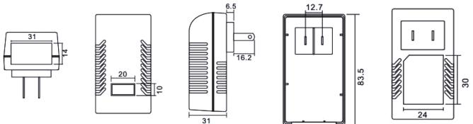
Wall mount PoE Injector and Power Supply
