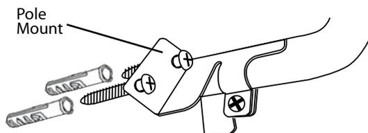
For wall mounting attach with bolts and wallplugs supplied on both sides of mount (far side not shown)
