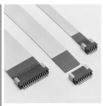
The FMS series connectors are designed for surface mounting (SMT) and to meet the demand for high-density packaging. They are miniature connectors with a height of only 2.8mm (.110"), and can be supplied packaged in embossed tape to facilitate automatic mounting.
