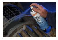
Cold Galvanising Spray is a unique combination of zinc powders and resins, formulated to form a high performance zinc-rich coating that actively fights rust and corrosion by its galvanic properties. Ferrous metals are protected by the sacrificial action, even when scratched or damaged. Zinc becomes the anode which is attacked by corrosion and the base metal the cathode. A film of waterinsoluble zinc oxide is formed, which stops rust and corrosion.
