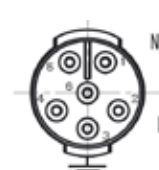
8MF1-PSM L: 85-264 VAC 4, 5, 6: Not connected
